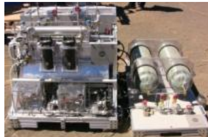
Water Electrolysis & Gas Storage
